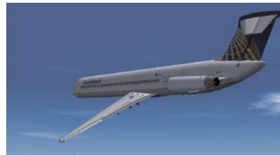
The DC9 (MD80) family is immediately recognisable by the long 'pencil' fuselage with rear-mounted twin engines
